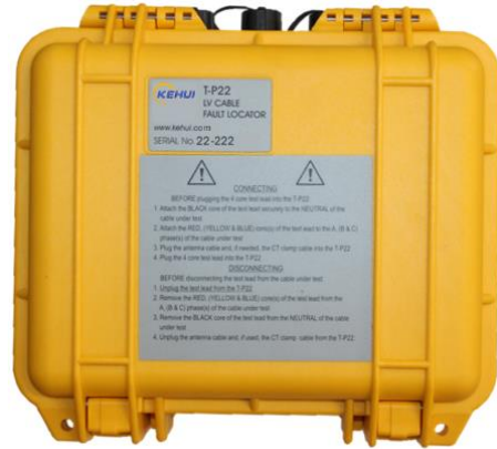
Figure 6.9: Connection and disconnection instructions on T-P22
