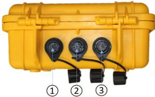
Figure 6.4: T-P22 terminals: ① Current clamp; ② Voltage connections; ③ Aerial
