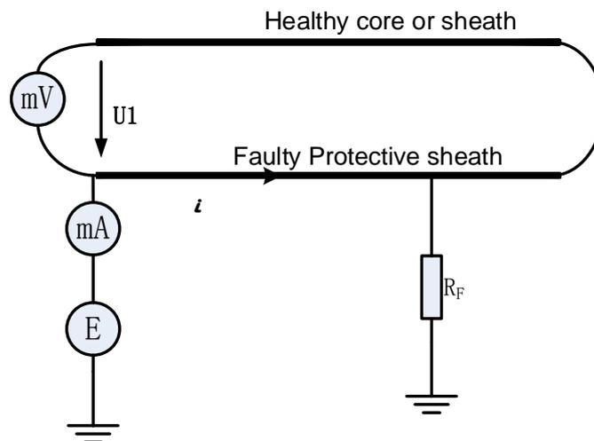
Figure 3.1 - DC Resistance method for sheath fault
