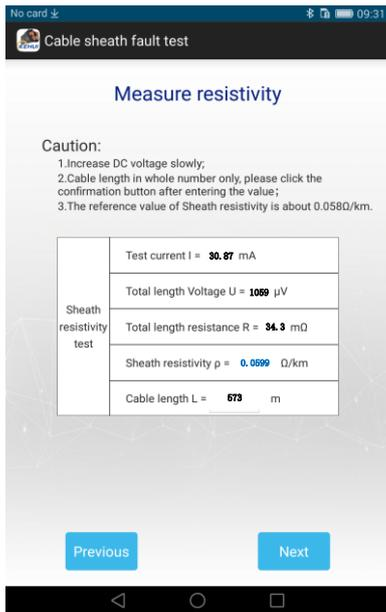
Figure 4.14 – Resistivity measurement screenshot
