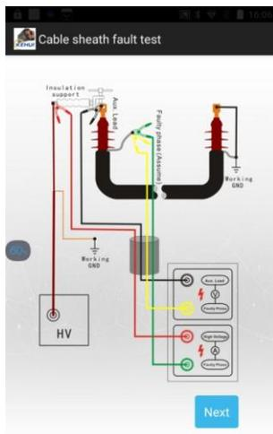
Figure 4.12 – Cable sheath fault test
