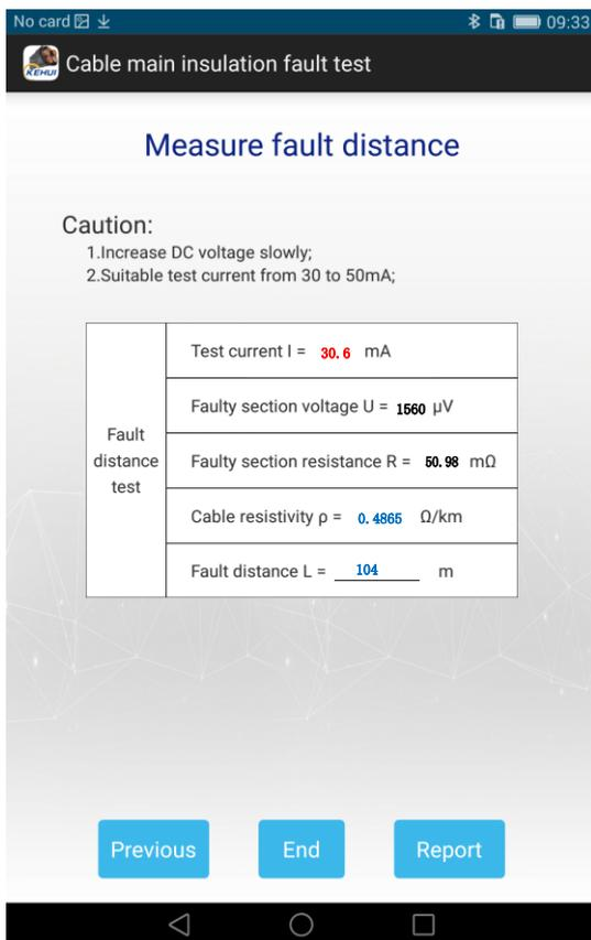
Figure 4.21 - Main insulation fault distance calculations
