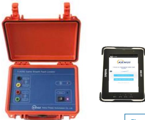
Figure 2.1 – T-H200 unit and tablet controller
