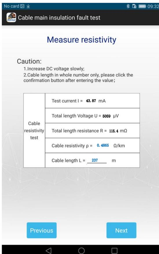
Figure 4.19 - Resistivity measurements
