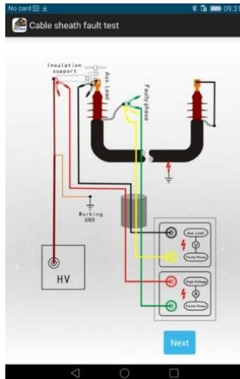
Figure 4.16 – Cable sheath fault location connection
