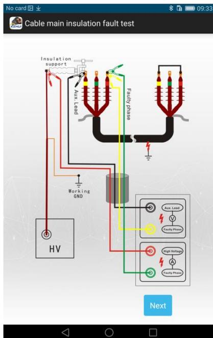
Figure 4.20 - Main insulation failure test connection diagram
