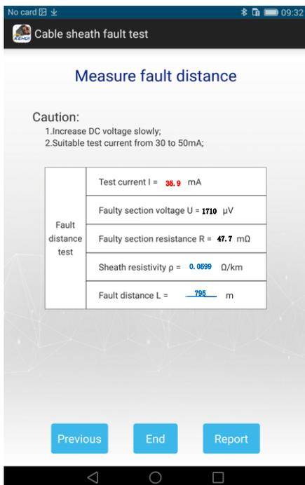
Figure 4.17 - Fault distance measurement
