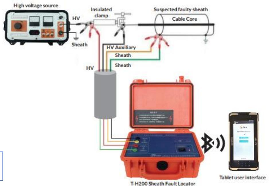
Figure 4.13 – Cable sheath fault test showing actual equipment
