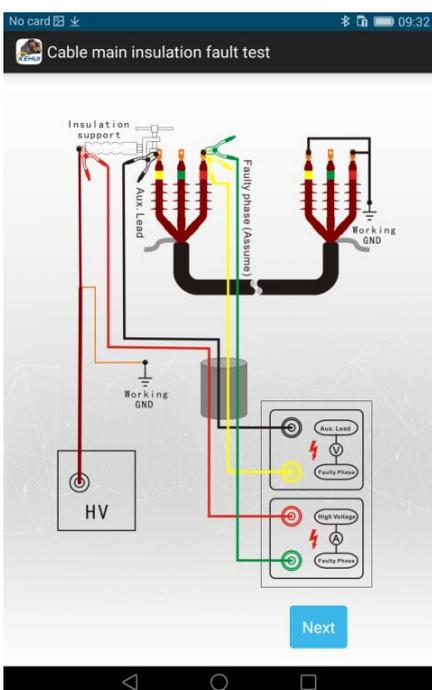
Figure 4.18 - Main insulation resistivity test connection diagram
