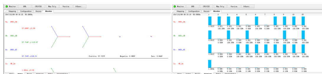
Figure 12.2-2 Real-time phasor information and harmonics
