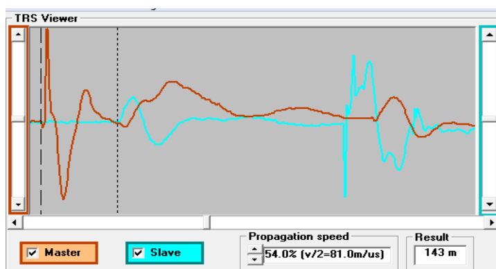
Figure 9.9a: fault location from the 'Master' end
