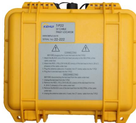
Figure 6.9: Connection and disconnection instructions on T-P22
