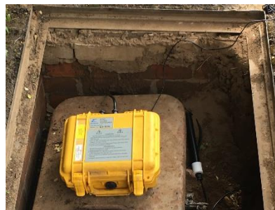
Figure 6.12b: T-P22 laid on top of the link-box bell housing
