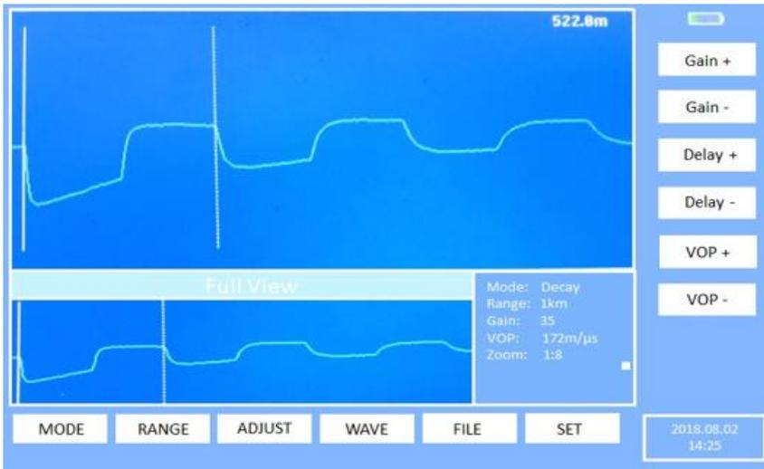
Figure 9-9 Decay method waveform showing the cursor at the reflection point
