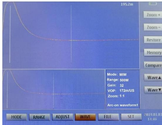
Figure 9-5 Multiple Impulse Method trace on the T-906 screen
