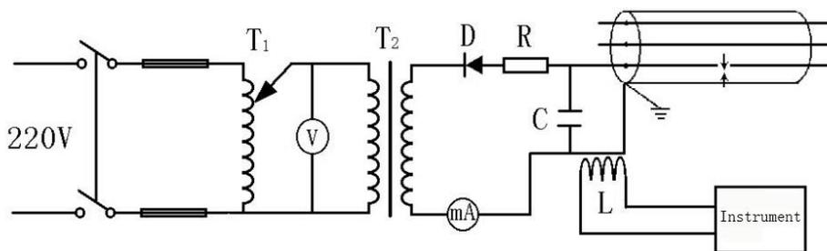
Figure 3-5 Set-up for DC flashover method
