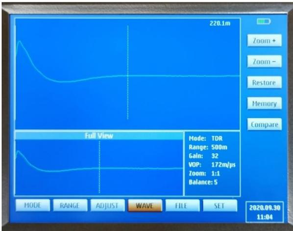
Figure 5-1: T-906 screen showing <wave> submenu.
