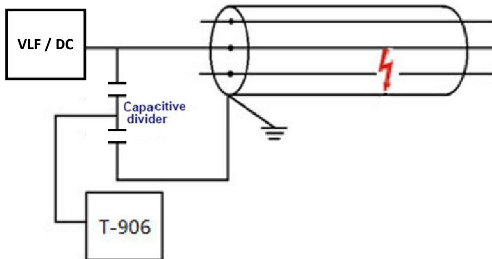
Figure 3-9 Set-up for the decay method
