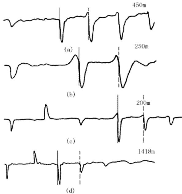
Figure 3-8 Waveforms for Impulse Flashover Method
