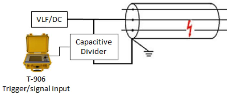
Figure 9-8 Set-up for the decay method
