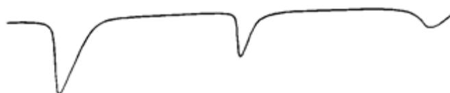
Figure 3-6 Waveform for DC flashover method
