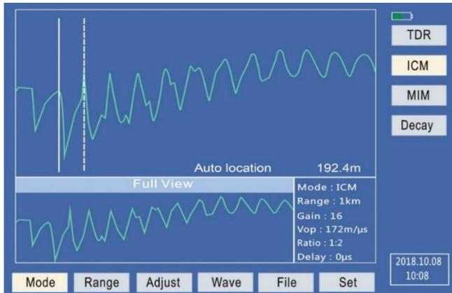
Figure 9-7 Automatic fault location for the ICM method
