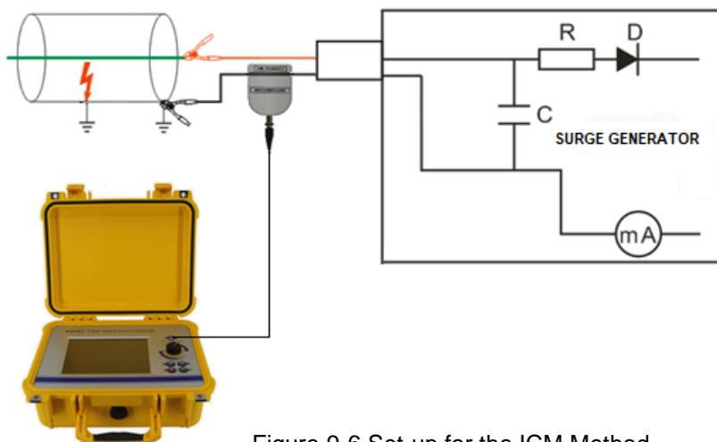
Figure 9-6 Set-up for the ICM Method
