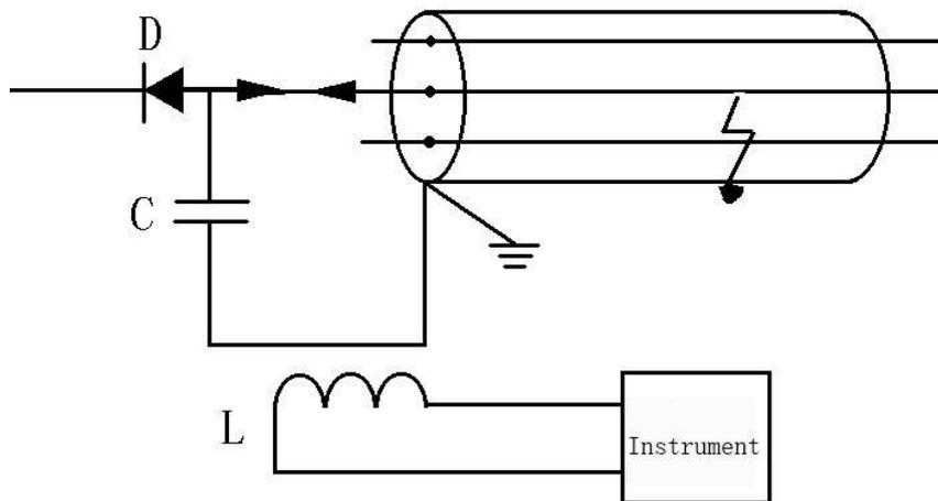
Figure 3-4 Set-up for Impulse Current Method
