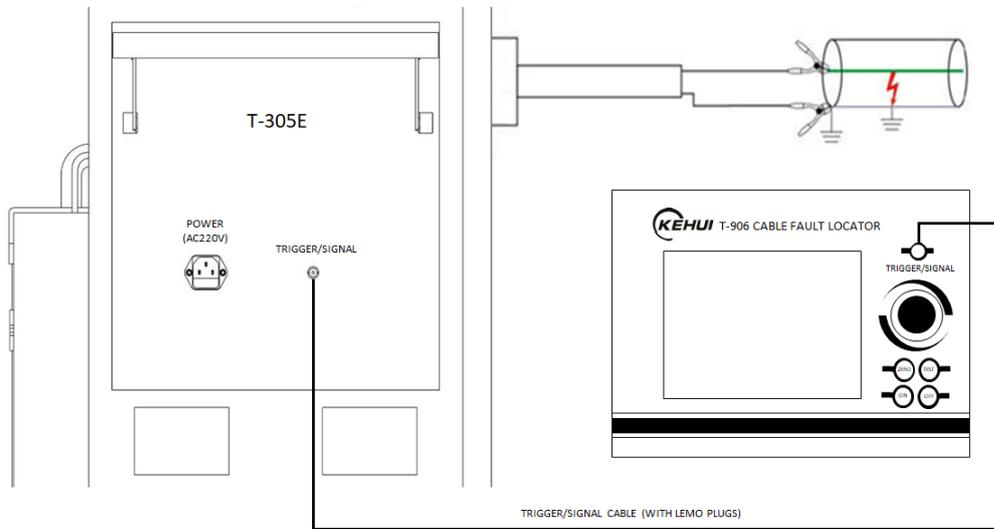
Figure 9-4 SIM/MIM set-up with T-305E
