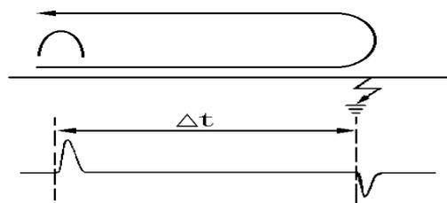
Figure 3-2 Round-trip time of reflected wave
