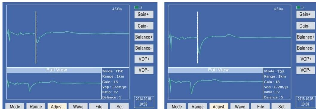
Figure 9-1 Gain adjustment of the TDR method
