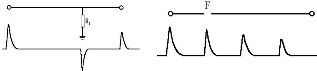
Figure 3-1 Reflected waves for short-circuit and open-circuit cable faults
