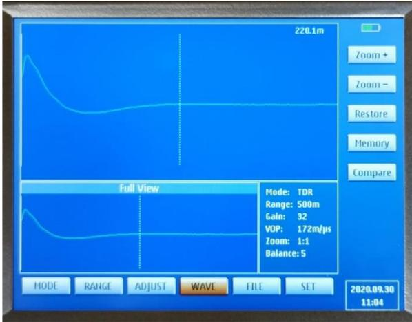
Figure 5-1: T-906 screen showing <wave> submenu.
