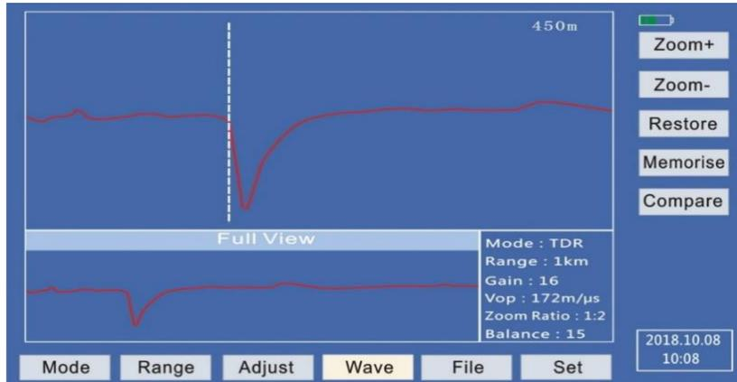
Figure 9-2 Zoom adjustment of the TDR method
